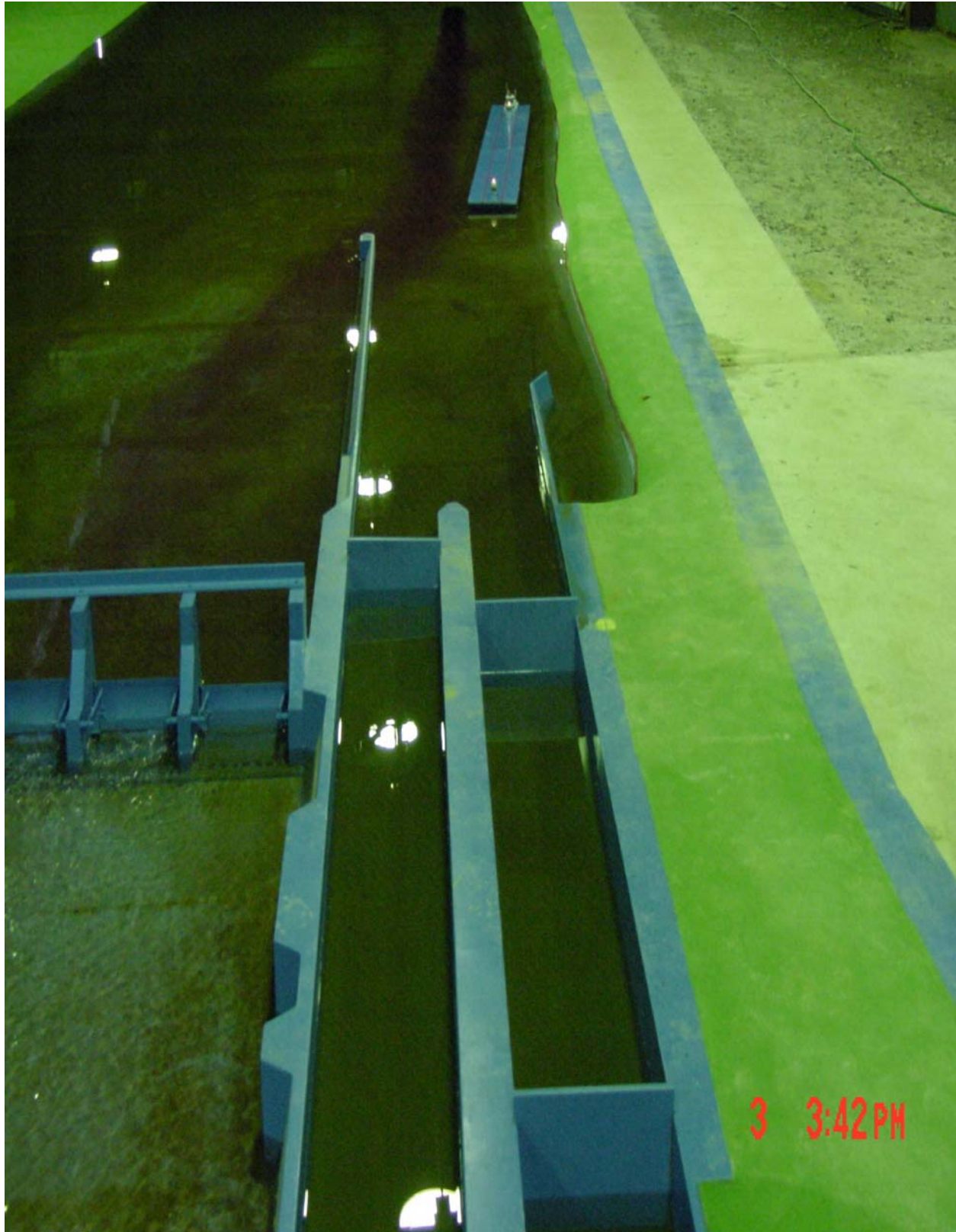
Figure B-8. Scale navigation model of Greenup L&D used for impact testing (Note: Scale model barge with tracking lights approaching the upper guard wall in top of photograph)
