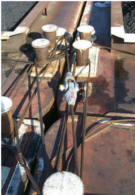
Figure B-3. Deck lashing (from Patev, Barker, and Koestler 2003a)
